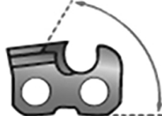
top plate cutting angle
