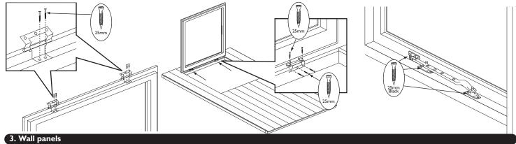
Position a large panel and a small side panel on the floor as shown. Note how the panel frames sit on the floor with the panel cladding overhanging the floor edge. Ensure square and secure using 3 x 50mm screws, screw through the frame of the small side panel into the frame of the back panel. Continue to add the remaining panels in the same way, in the order shown below.
